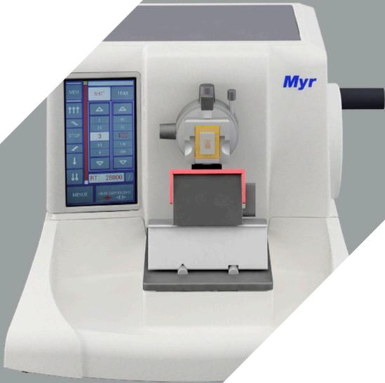
Automatic fixation of the **knife carrier** to the microtome base (patent pending) and removable lever for locking the clearance angle of the blade holder. Design without levers for improved cleanliness and ease of use. Blade holder can be moved sideways both to the right and the left for an optimal use of the cutting edge.
