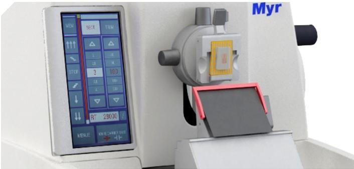
Equipped with a **specimen orientation head** that works with different specimen clamp types and an easy-to-operate change system thanks to the blocking mechanism. Indication of 0-position in x and y direction by palpable click for the precise position of the specimen. Cutting-edge design of the specimen clamp that prevents building up of dirt and facilitates operations with the microtome.
