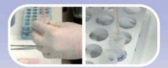
4 Add 6-10 drops of liquid Bio-Agar to the sample on the vial's bottom
