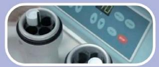
2 Centrifuge the sample for 10 minutes at 2500 RPM
